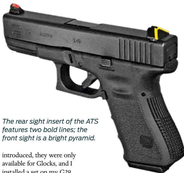
*The rear sight insert of the ATS features two bold lines; the front sight is a bright pyramid.*
