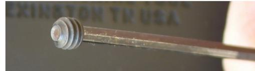
IF a second set of 1/8" screws is included: After firmly seating set screws, install 1/8" lock screws on top to lock them in place. **Do not use threadlocker on these screws. There is no need and too much risk of getting threadlocker inside body.**
