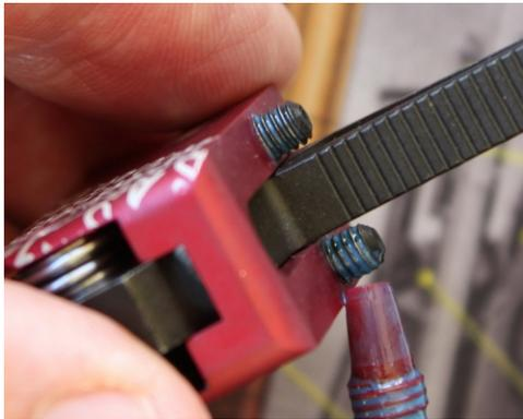
Prepare trigger by turning set screws out about 3/16" & placing a **very** small amount of blue threadlocker on threads.
