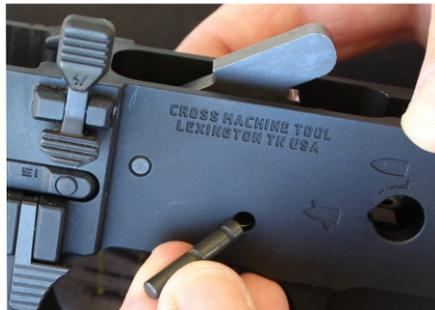
Drop in ELF trigger and replace pins
