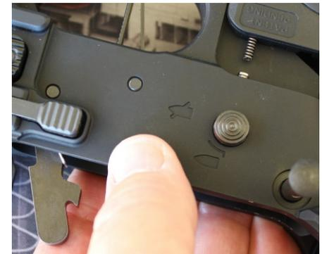
With hammer in "half cock" position, insert safety and grip with safety detent and spring in place.
