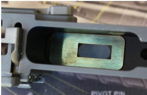
Insert steel floorplate to protect receiver (Wider end forward)
