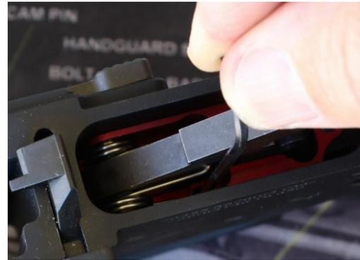
Center the pins in the receiver and firmly seat the two set screws on the inside of the trigger body. It is absolutely critical that these screws are seated firmly even if anti-walk pins are used. Turn each side until it just touches, then alternate so the pressure is evenly distributed.
