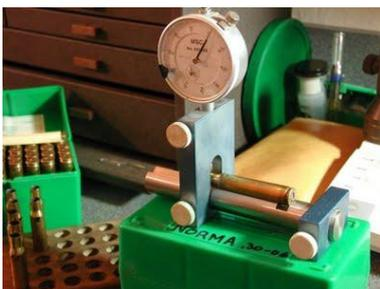
**diameter and loaded brass is 0.333" diameter**, so there is a fair amount of work to be done in sizing and necks do not maintain perfect concentricity through the process.
