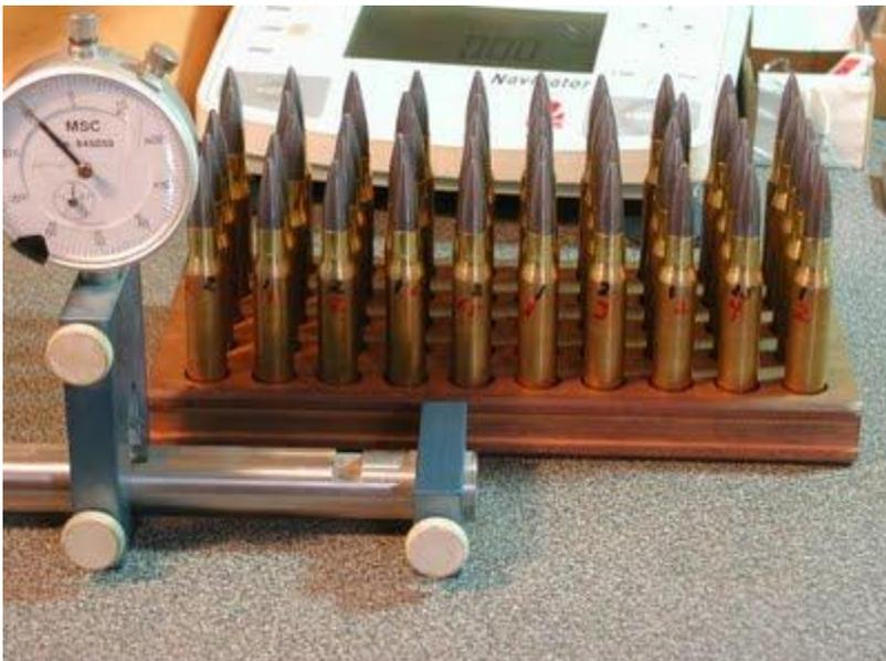
Once the bullets were seated, I reset the concentricity tool to **measure runout right at the ogive of the bullet**. I think this is the critical point as it will contact the rifling first and will determine the bullet's initial squareness to the bore.
